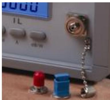
This connector of power meter is also movable. When it is not in operation, please cover the dust-cap to keep it clean
