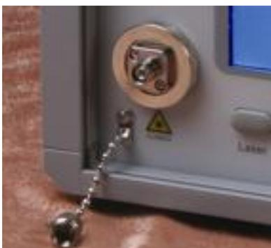
This connector of light source is movable and easy to be cleaned.
